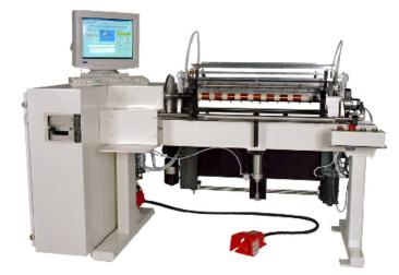
The Model 307 stick winder is a recent design that is based on the industry standard Leesona 107. It is greatly improved with a PC based MCS4 control and a combination of servomotors and air operated devices. The machine is fully programmable on all functions related to winding and paper feeding.
